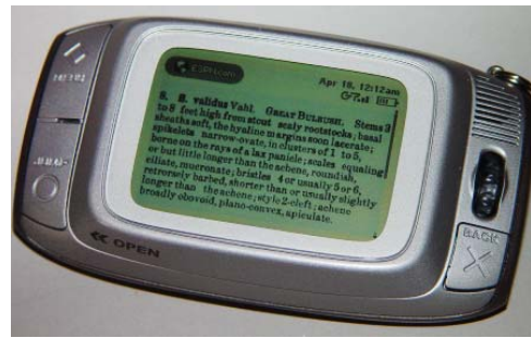
Figure 5. Display of reflowable images on the Danger Hiptop, a cell phone with a screen resolution of 240 \times 160 .
