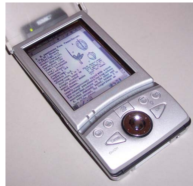
Figure 4. Display of reflowable images on a Sharp Zaurus at 240 × 320 pixels.
